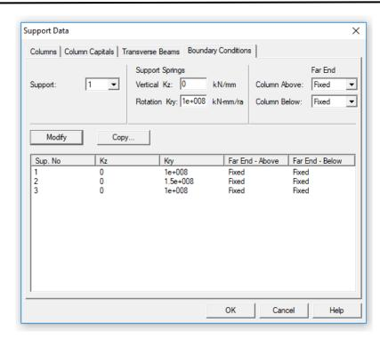
Figure 18 - Beam Supported by Transverse Beams - Defining Supports Stiffnesses (spBeam)
