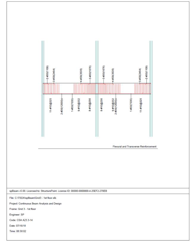
Figure 15 - Longitudinal and Lateral Reinforcement (spBeam)
