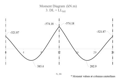
Figure 8 - Maximum Moments for the Total Service Load Level
