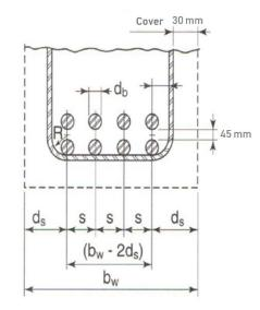
Figure 6 - Maximum number of bars in beams
