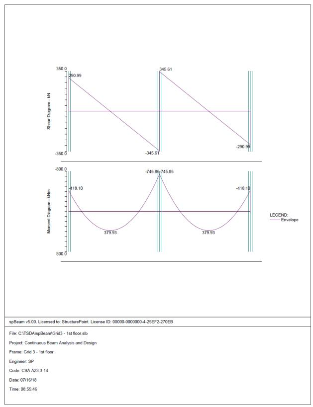
Figure 11 – Internal Forces (spBeam)
