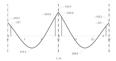
$\frac{500}{1000} = 0.5 \text{ m} < 0.175 \times 12 = 2.1 \text{ m} \text{ (use face of supporting location for interior column)}$
