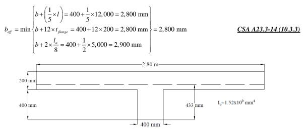
Figure 3 - Moment of inertia calculation for T-beam section
