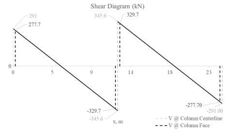
From the following Figure, the shear value in end span at face of the interior support governs.
