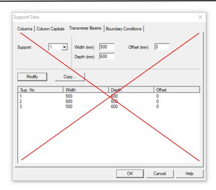
Figure 17 – Beam Supported by Transverse Beams – Defining Supports Geometry for two-way Slab systems (spBeam)
