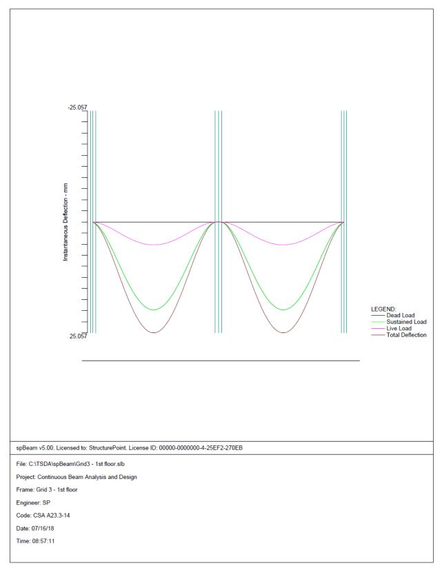
Figure 14 – Immediate Deflection Diagram (spBeam)
