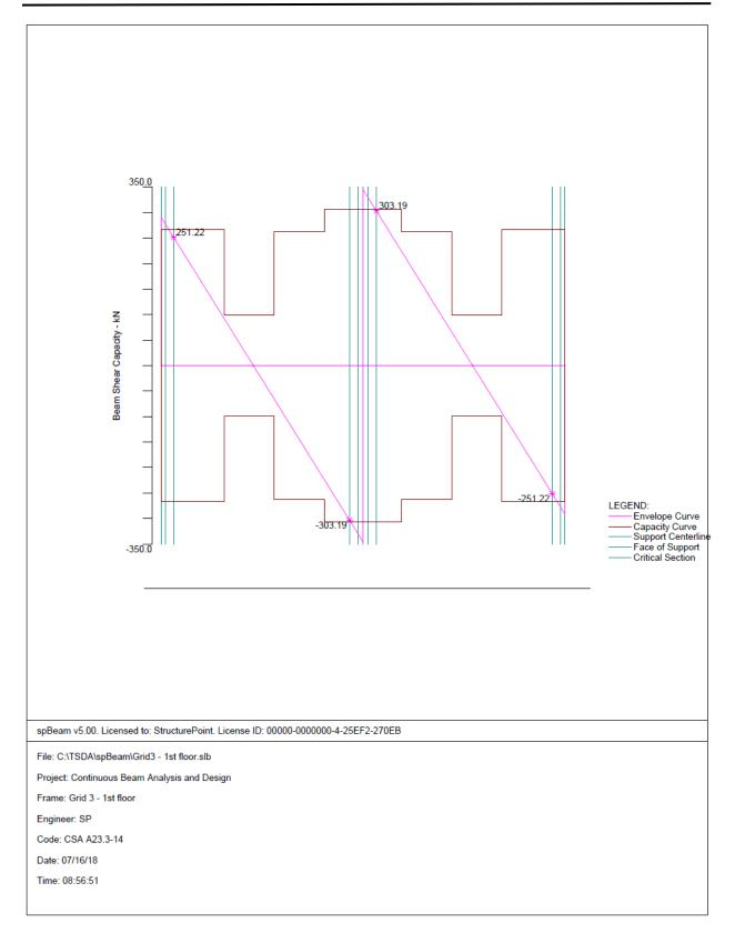
Figure 13 – Shear Capacity Diagram (spBeam)
